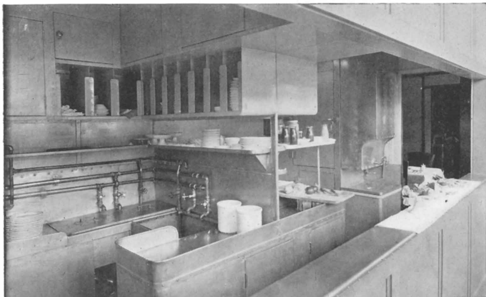
One end of the kitchen and pantry of the Training School and Experimental Kitchen. The door-way to the right is the entrance to the dining compartment. The arrangement in space and equipment is exactly the same as that on a dining-car in actual operation
